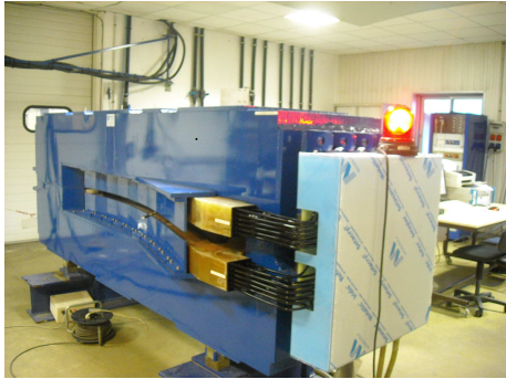
Figure 11: Prototype spiral FFAG magnet, under measurement at SigmaPhi.
