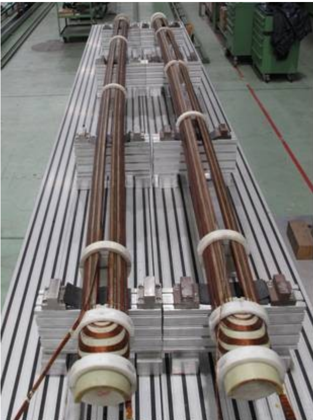
Fig.3: Two complete poles, after curing,
