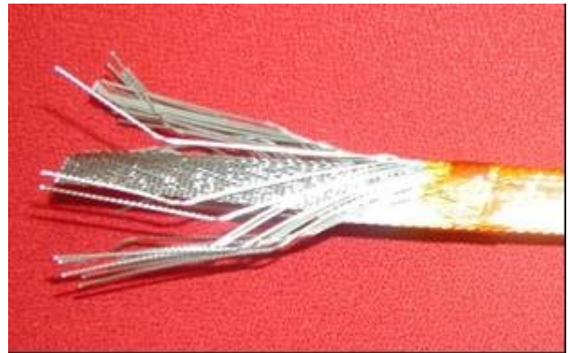
Fig.5: The trial winding conductor used for the winding tests. In between the strands one can see the thin stainless steel core used for depressing the inter-strand coupling currents.
