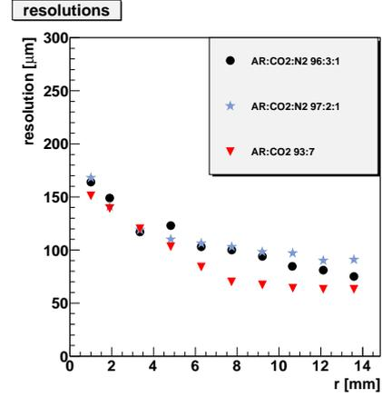
Figure 2: Single tube resolution of the standard gas (triangles) and two gas mixtures (stars and circles) containing 1%  $\text{N}_2$
