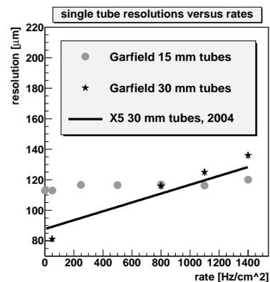
Figure 7: Comparison of simulated (circles and stars) and actual (line) to measured resolutions of 30 mm tubes.
