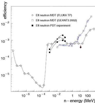
Figure 5: Different simulations of neutron efficiency [7]. Our result is the data point at 11 MeV and  $4 \cdot 10^{-4}$ .
