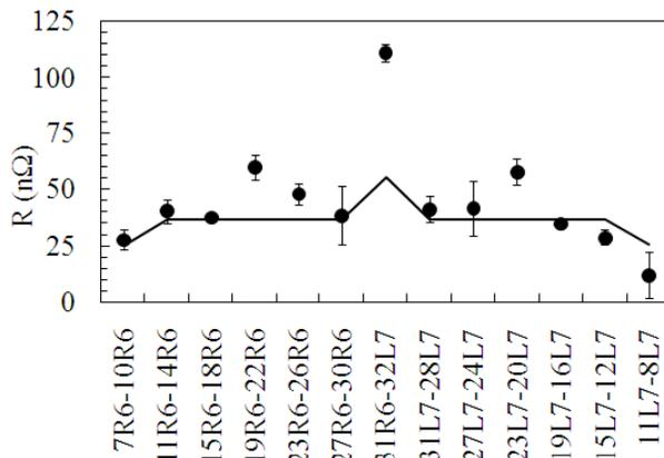
Figure 2: Total resistance in the dipole circuit in each sub-sector in sector 67, measured by the calorimetric method.
