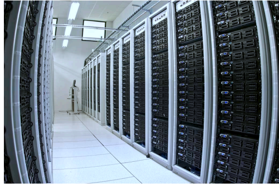
Figure 9. Racks of Dell PE 2850 and PE 1950 computers used for the event building and for the high-level triggers.
