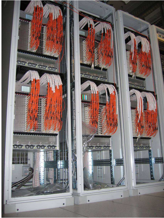
Figure 7. 72 crates holding 8 \times 8 Myrinet switches used for the FED builder located close to the event builder and high-level trigger farm.
