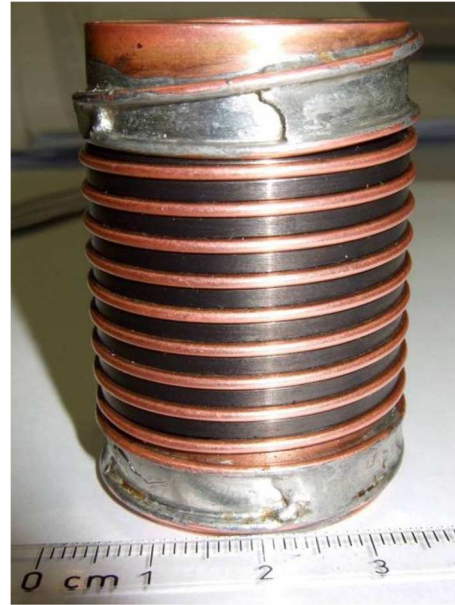
Fig. 3. Sample holder for critical current measurements of \text{Nb}_3\text{Sn} superconducting strands. The PIT strand is wound onto a grooved Ti-6Al-4V cylinder with an outer diameter of 32 mm. After the reaction HT the wire is soldered onto Cu cylinders at both ends of the barrel.
