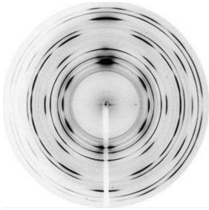
Fig. 2. Debye-Scherrer diffraction pattern of a reacted \text{Nb}_3\text{Sn} strand acquired in transmission geometry with a MAR 345 image plate detector.
