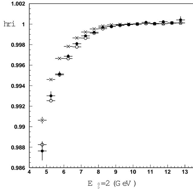
Fig. 9. Average  $\langle r \rangle = m_0 = m_0$  versus  $E_0 = 2$  for  $\pi^0$  pairs from  $K^0 \rightarrow \pi^0 \pi^0$  decays selected as described in the text. Solid circles: data; crosses: simulated events; open circles: simulated events corrected for non-linearity (see text). The  $m_0$  energy is divided by 2 to compare with the energy for symmetric  $\pi^0 \rightarrow \pi^0 \pi^0$  decays.
