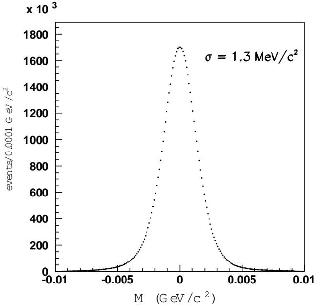
Fig. 2. Distribution of the difference between the invariant mass and the nominal  $K^0$  mass for the selected  $K^0 \rightarrow \pi^0 \pi^0$  decays.
