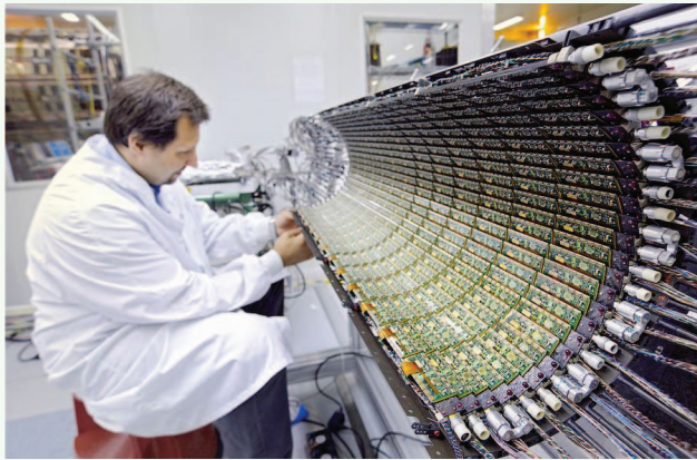
Fig. 7 Final assembly work on the Atlas pixel barrel (half). One can see the modules along the ladders. The white stubs are connecting tubes for the cooling channels, one for each ladder. Photo CERN/Atlas.
