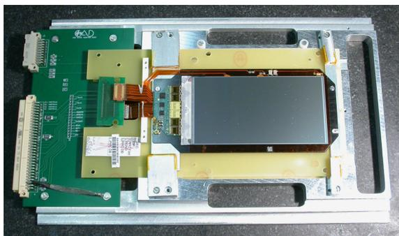
Figure 2: TIB Layer 3 module mounted on the aluminium test plate and connected to interface cards.
