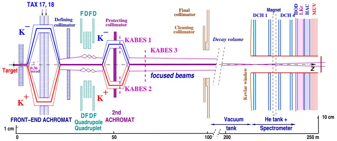
Figure 1: Schematic lateral view of the NA 48/2 beam line (TAX 17,18: motorized beam dump/collimators used to select the momentum of the  $K^+$  and  $K^-$  beams; DFDF/DFDF: focusing set of quadrupoles, KABES1{3: beam spectrometer stations not used in this analysis), decay volume, and detector (DCH1{4: drift chambers, HOD: hodoscope, LKr: EM calorimeter, HAC: hadron calorimeter, MUV: muon veto). Note that the vertical scales are different in the two parts of the figure.
