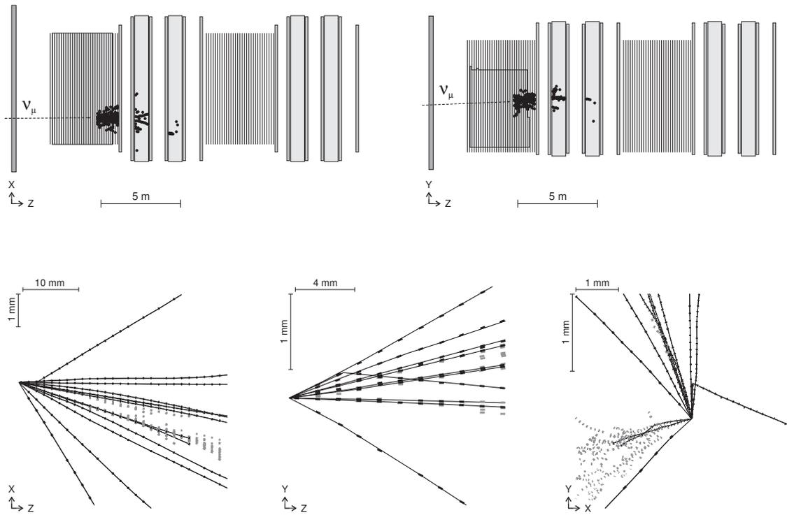
Figure 13: Online display of the OPERA electronic detector of a charged-current interaction with a charm-like topology (top panel). The reconstruction is shown in the bottom panels where the charm-like topology is seen as a track with a kink: top view (bottom left), side view (bottom center), frontal view (bottom right).
