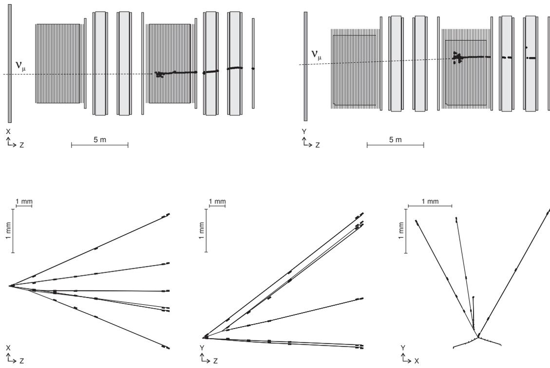
Figure 14: Online display of the OPERA electronic detector of a charm-like topology (top panel). The emulsion reconstruction is shown in the bottom panels where the charm-like topology is seen as a three-pronged secondary vertex: top view (bottom left), side view (bottom center), frontal view (bottom right).
