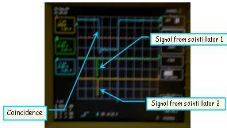
Figure 4: Three coincidence signals from two scintillator planes and a chamber.
