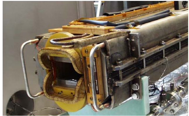
Figure 15: 4KDP6a dipole (connection side).
