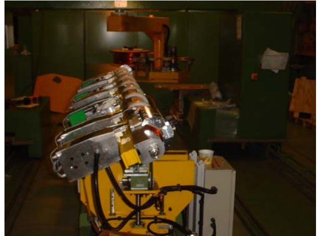
Figure 5: Winding operations with dummy cable
