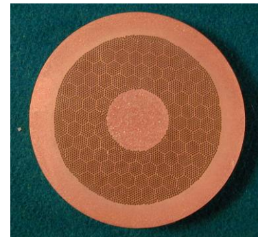
Figure 3: The Nb-Ti strand for ITER PF1&6 coils. Strand diameter: 0.73 mm, Cu/nonCu ratio: 1.6, filament diameter: 6.8 \mu\text{m} .
