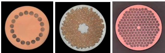
Figure 1: The Nb-Ti strands for different applications: a) for MRI tomographs, b) for AC electro technical devices, c) Strand for accelerator UNK (CKHT-8910-042).
