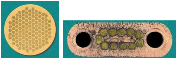
Figure 8: Left: Cross section of the Non stabilized bronze processed strand 1.5 mm in diameter; number of filaments: 14641; filaments diameter: 5 μm; J_c @ 8 T: 510 A/mm 2 ; average I_c : 900 A. Right: cross section of conductor for T-15; critical current @ 8 T is ~ 11.5 kA, i.e., ~ 110% of single strands current ability (11×900 A).
