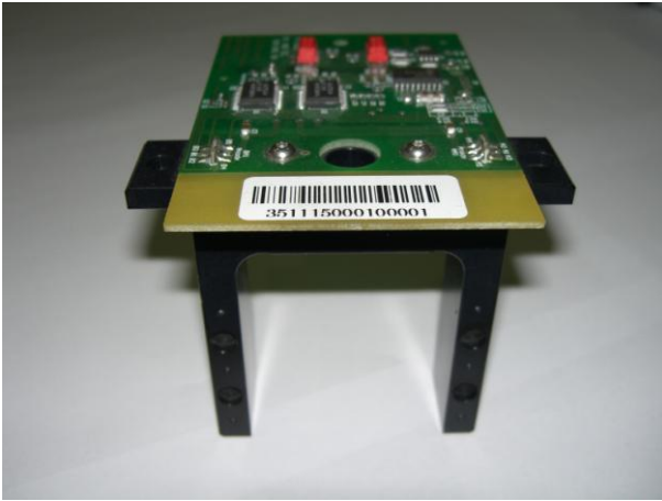
Figure 3: Barrel Fork. Each of these elements contain 10 LEDs. Four of these forks are mounted on each of the 250 DTs.
