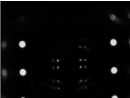
Figure 8: On this real image not every spot of the closer fork can be seen. Discarding un-observable direct spots helps to minimize errors arising from false spot measurements.
