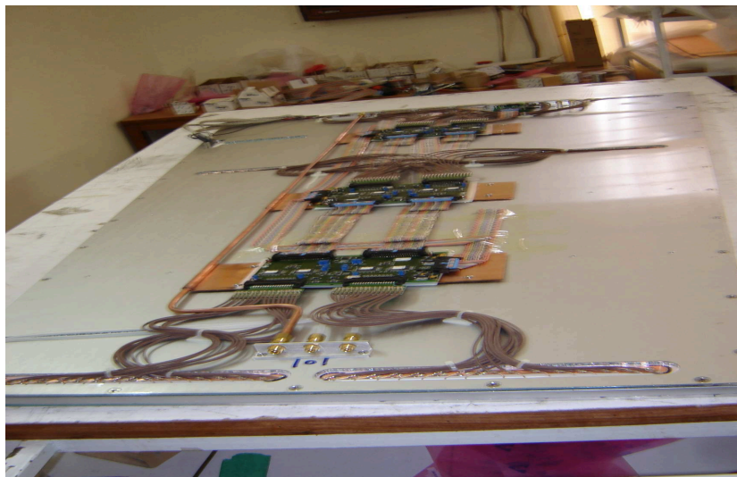
Figure 3: Readout electronics and cooling system of chamber.
