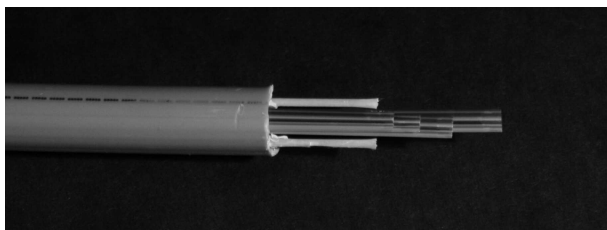
Figure 41. Photograph of an optical cable used for transmitting FEB digital readout data from the FEC to the BE electronics. The fiber ribbons are visible emerging from the outer protective sheath.
