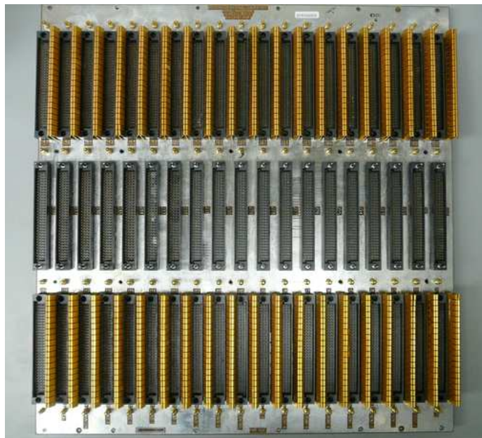
Figure 40. Photograph of a FEC baseplane for the EMB. The upper and lower rows of connectors are used for input signal connections to the FEBs, and are surrounded by custom springs for improved grounding. The middle row is used for connecting the L1 sums from the FEBs to the TBB/TDB.
