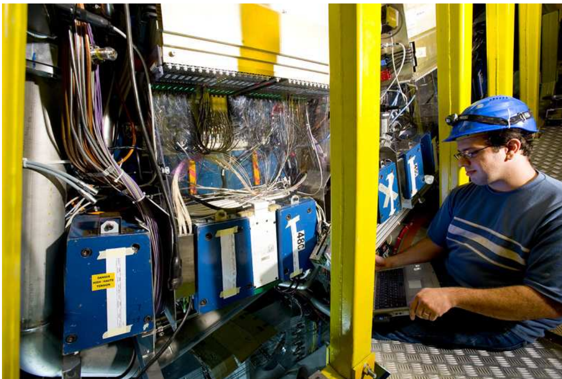
Figure 27. Photograph of a LVPS and FEC installed on the ATLAS detector and being commissioned. The LVPS is the white box visible toward the bottom of the photograph, while the FEC is visible above the LVPS.
