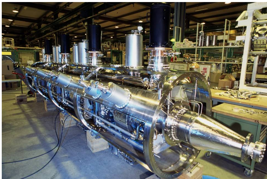
Figure 4.2: Four-cavity module during assembly.
