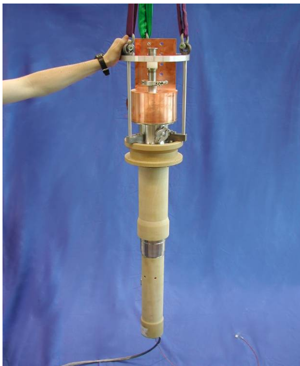
Figure 6.5: 13 kA CERN prototype HTS current lead.
