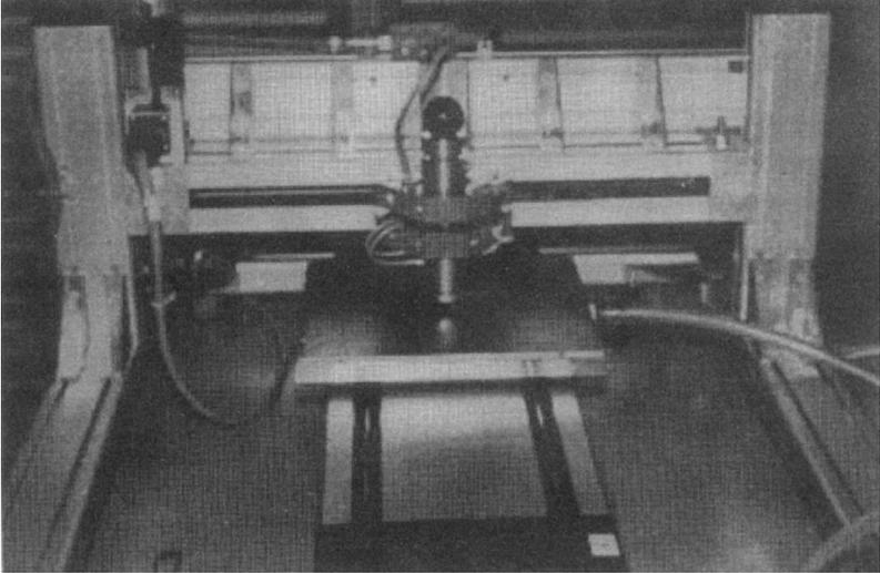
FIGURE 14 Eddy current scanning apparatus for quality control of Nb sheets.
