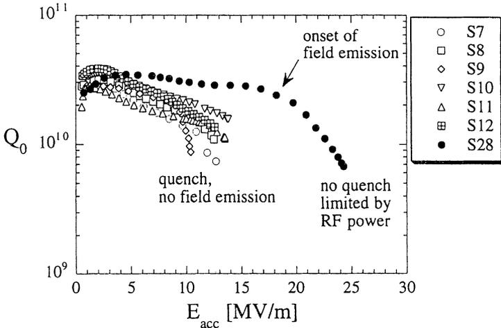
FIGURE 4 Performance of 6 cavities from one vendor: decrease of the  $Q$  value at low gradients (but *no* field emission) and early thermal breakdown between  $E_{acc}$  10 and 14 MV/m. The defects were localised at the equatorial welding and could be traced back to improper cleaning and not optimised welding parameters. One more cavity was fabricated with improved fabrication conditions and showed excellent performance (S28).
