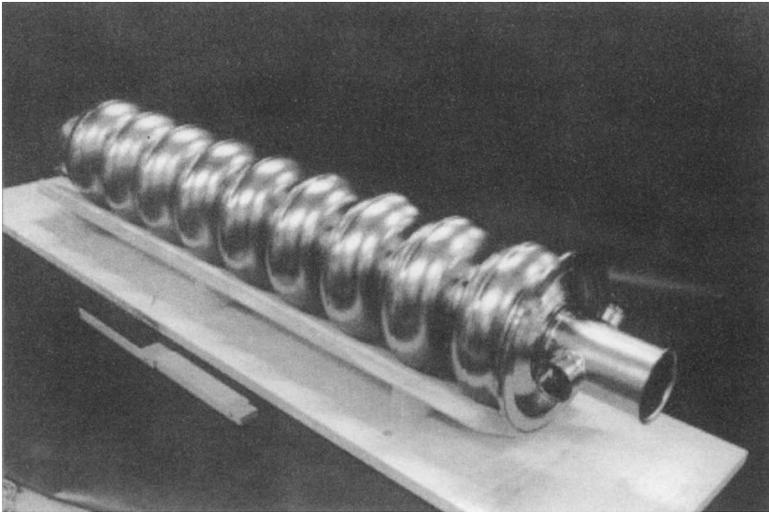
FIGURE 2 Nine-cell TTF cavity. On the right beam pipe the port for the input coupler (front side) and the HOM coupler (back side) can be seen.
