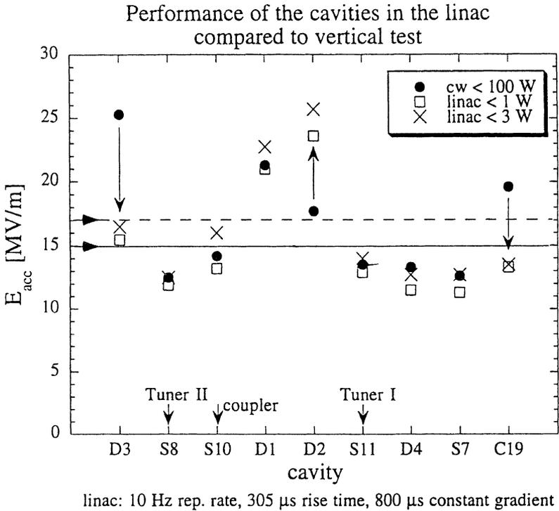
FIGURE 11 Performance of the cavities in vertical tests (dark circle) and in the linac module (cross, open square). The gradient  $E_{acc}$  is noted just below thermal breakdown or at the onset of field emission. The cavity D2 upgraded in the linac operation because the time constant of the thermal breakdown is longer than the linac RF pulse. Cavities D3 and C19 degraded because of enhanced field emission.
