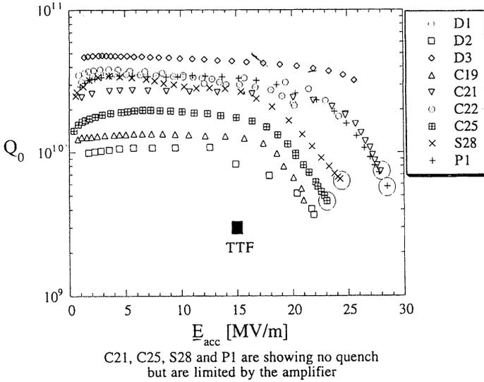
FIGURE 3 Performance of “good” cavities in the vertical measurement. Four cavities (C21, C25, S28, P1) were limited by available RF power. The typical decrease of the  $Q$  value at high gradients is due to field emission.
