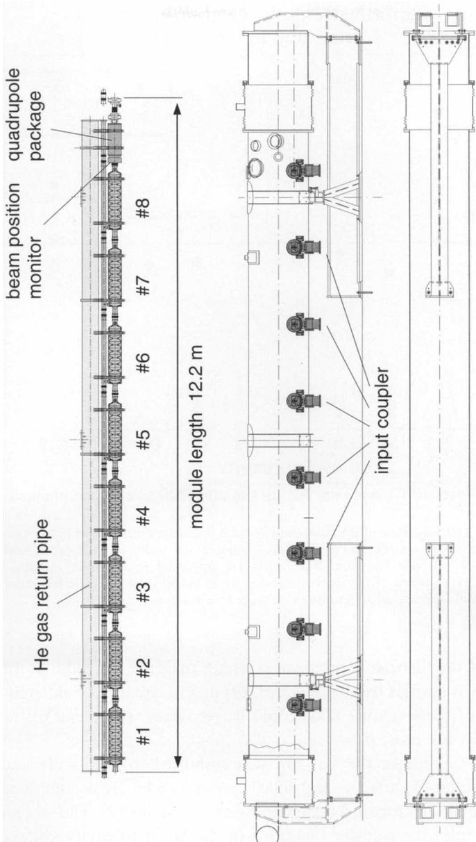
FIGURE 10 Longitudinal cut through one module (8 cavities, one quadrupole) of the TTF cryostat.
