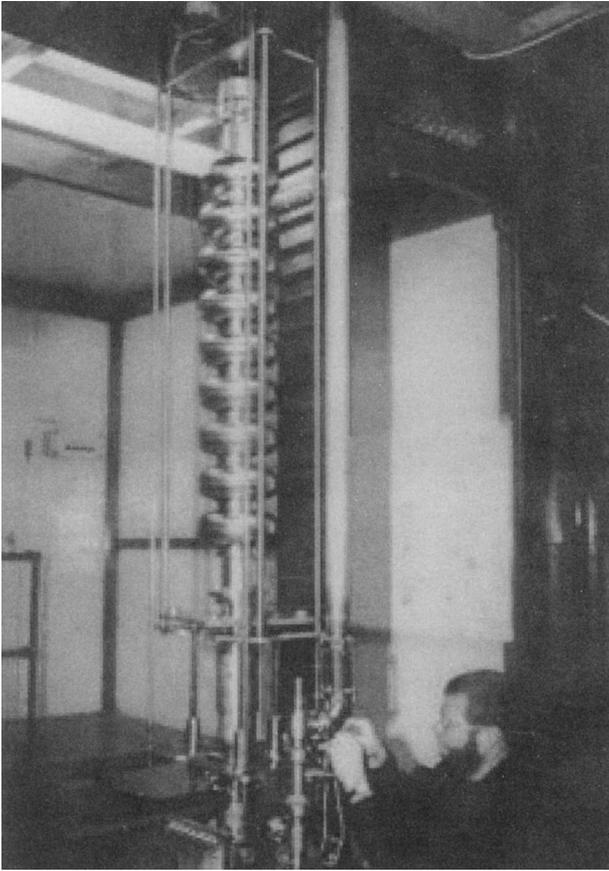
FIGURE 6 Vertical test stand for acceptance test of the nine-cell cavities. The rectangular waveguide parallel to the cavity will transport RF power for high power pulse processing (HPP).
