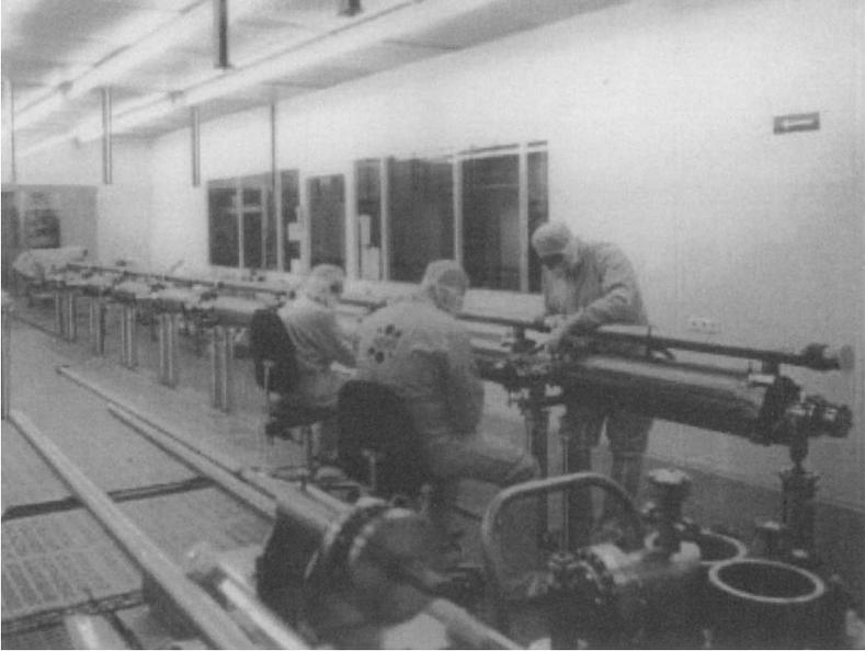
FIGURE 8 Assembly of a string of 8 nine-cell cavities and one quadrupole during handling in the clean room.
