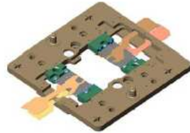
6. Blade A (with Bearings) & Blade B (without inserted) in turnplate
