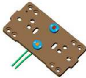
3. Chips transferred and held by vacuum
