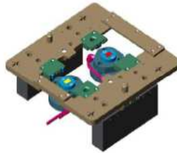
4. Invert turnplate. Repeat for chips 3&4
