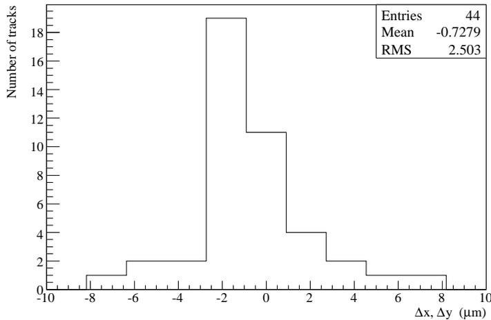
**Figure 18.** The distribution of the position residuals between CSd emulsion films after the local offset correction. A CSd track has two entries referring to the residuals for the X and Y projections.
