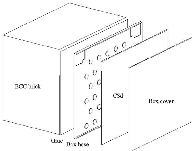
**Figure 6.** Mounting the CSd on the ECC brick.
