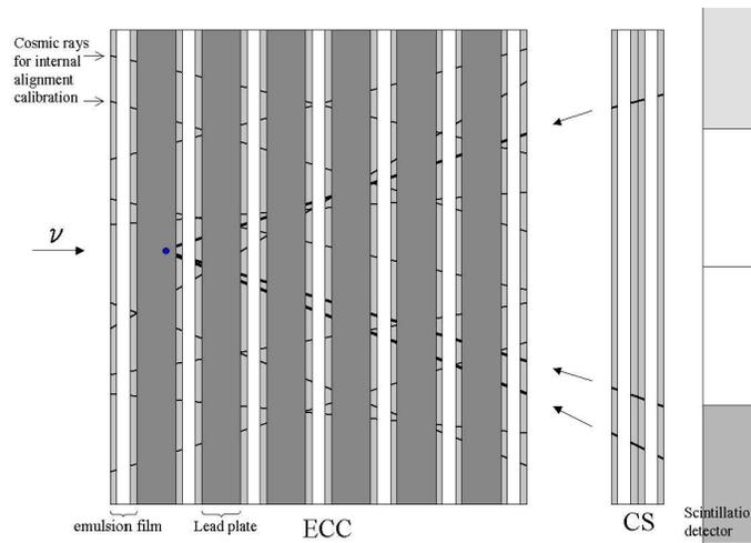
**Figure 3.** Schematics of the CS - Scan-back method.
