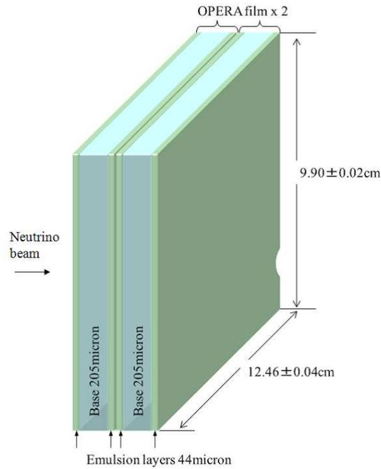
**Figure 2.** The schematic drawing of the CS doublet.
