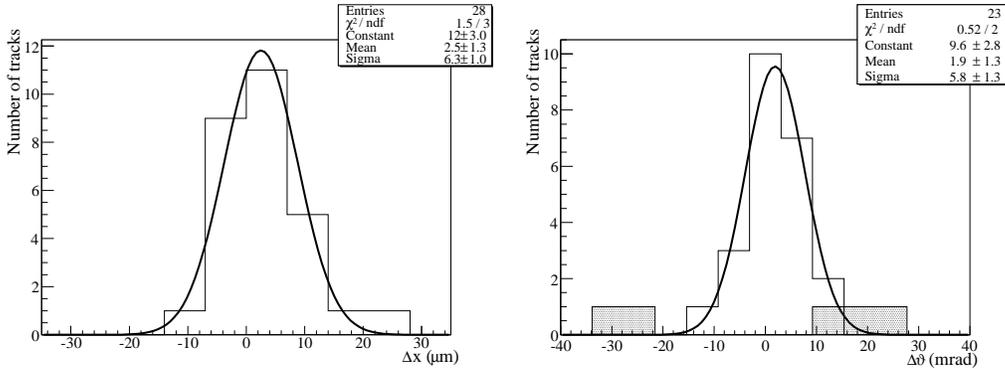
**Figure 14.** Distributions of the position and angular residuals between CSd emulsion films. For angular residuals open boxes refer to tracks formed by two base-tracks while filled boxes refer to tracks formed by a base-track and a single micro-track.
