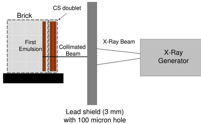
**Figure 12.** Schematic view of the X-ray system.
