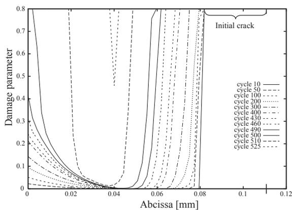
**FIGURE 4** Damage evolution across the wall thickness under cyclic loading
