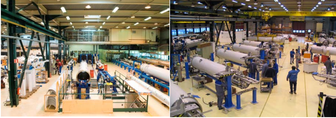
FIGURE 1. Views of the SSS assembly hall at CERN: Cryostat assembly benches (lefts), and Technical Service Modules assembly benches (right).
