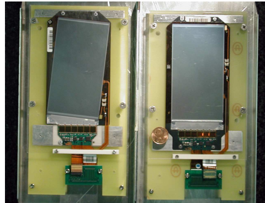
Figure 3: TIB modules in their module carrier. On the right side, a r- \phi module and on the left side, a stereo right module are shown.
