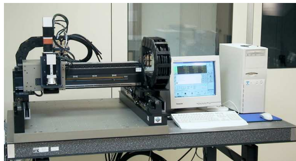
Figure 5: out-of-the-box Aerotech AGS 10000 system
