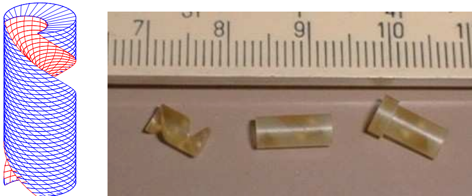
Figure 10. Wire support drawings and photos. In the photo: Left - a bare wire support (twister). Middle - embedded in a cylindrical sleeve as a centre wire support. Right - embedded in a flanged sleeve as an outer wire support.
