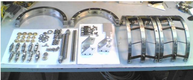
Fig. 7 – Tuner components before assembling
