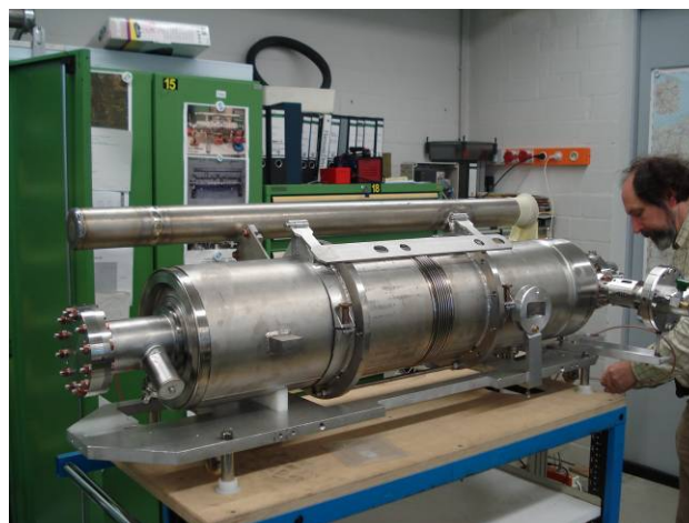
Fig. 6 - Cavity integrated in the modified helium tank in Halle III machine shop at DESY
