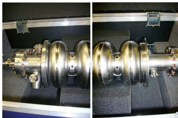
Fig. 5 - Z86 cavity after the rings EBW at Lufthansa facility
