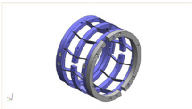
Fig. 4 - The additional adaptation rings, in grey, installed for the Slim tuner
