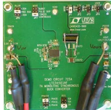
Figure 4: LTC3415E Evaluation Board with Air Coil
