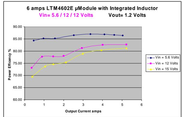
Figure 8: LTM4602V Power Efficiency with various input Voltages
