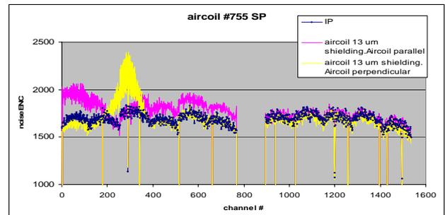
Figure 5: Noise Histogram from Silicon Sensor. Left plot is for top sensor facing the Air Coil. Right side plot is for the sensor below the top sensor.
