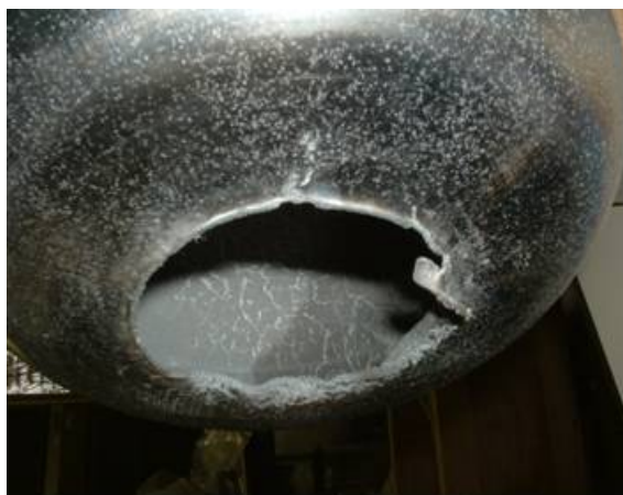
Fig. 3.2: Destroyed cavity after tumbling because of a too small wall thickness at the iris region The thickness uniformity experimentally found in this region is sketched in the next figure.
