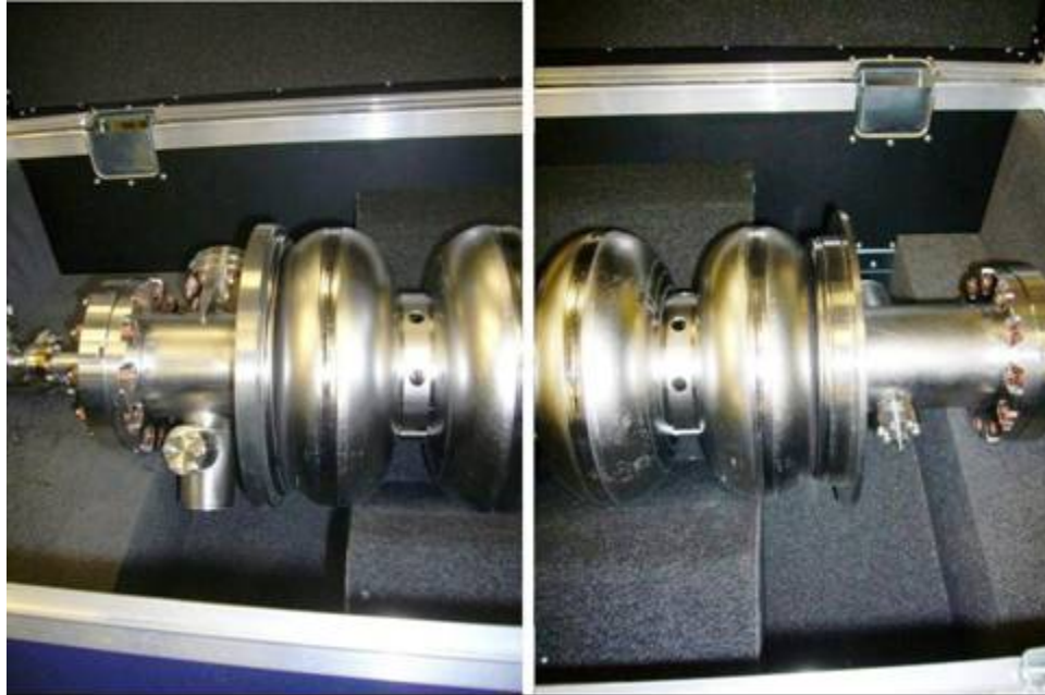
Figure 8. 1: Z86 cavity after the rings EBW at Lufthansa facility
