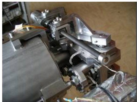
Fig.10.2 Magnetostrictive Actuator: mechanical part (left) – installation on a 9-cell cavity (right)
