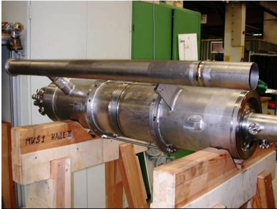
Figure8. 2: Cavity integrated in the modified helium tank in Halle III at DESY
