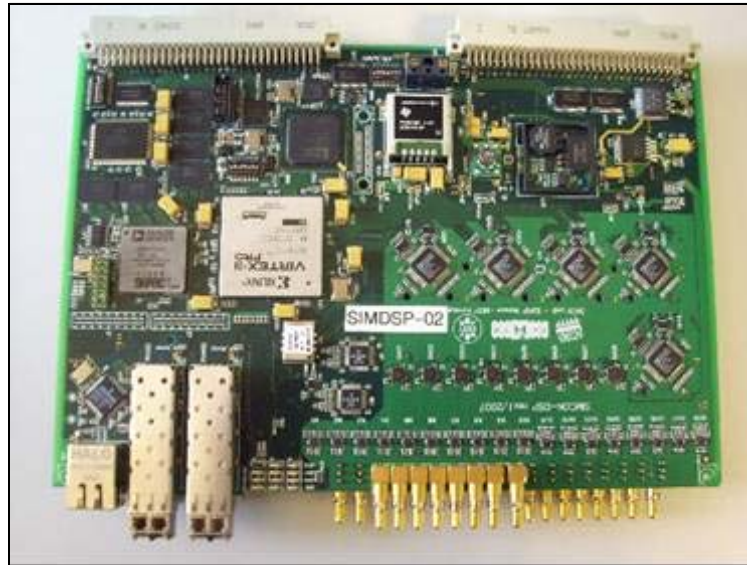
Figure 9.7 Debugged control board SIMCON DSP
