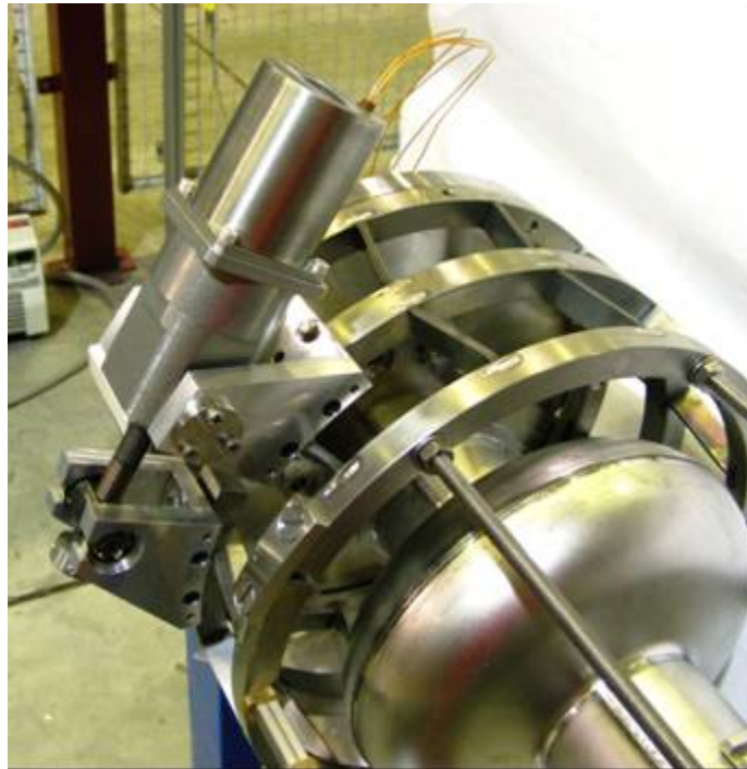
Figure 8. 4: the optimized coaxial tuner for ILC.
