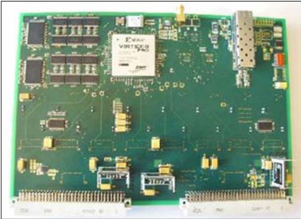
Figure 9.5 Digital motherboard suited to carry mezzanine boards with downconverters and ADC
