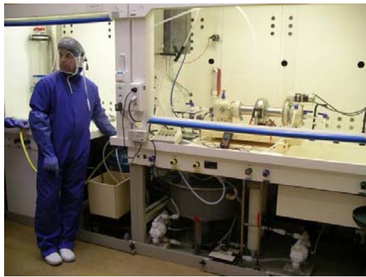
Fig. 5.1: Single cell electropolishing (EP) installation at Saclay.
