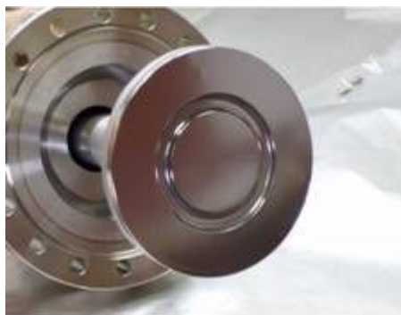
Fig.4.2.6. Large copper sample fixed upon an insulating support (just before the coating).
