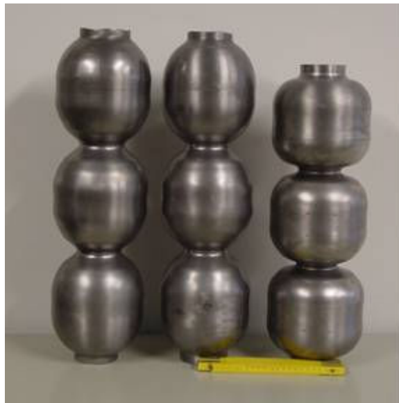
Fig. 3.2.4: Example necking of the niobium three cell unit.
