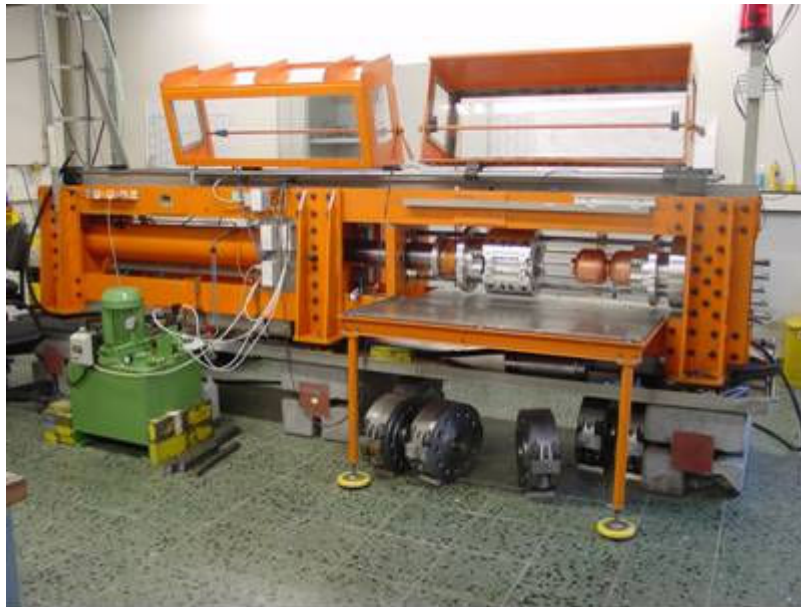
Fig. 3.2.6: View of the hydroforming machine
