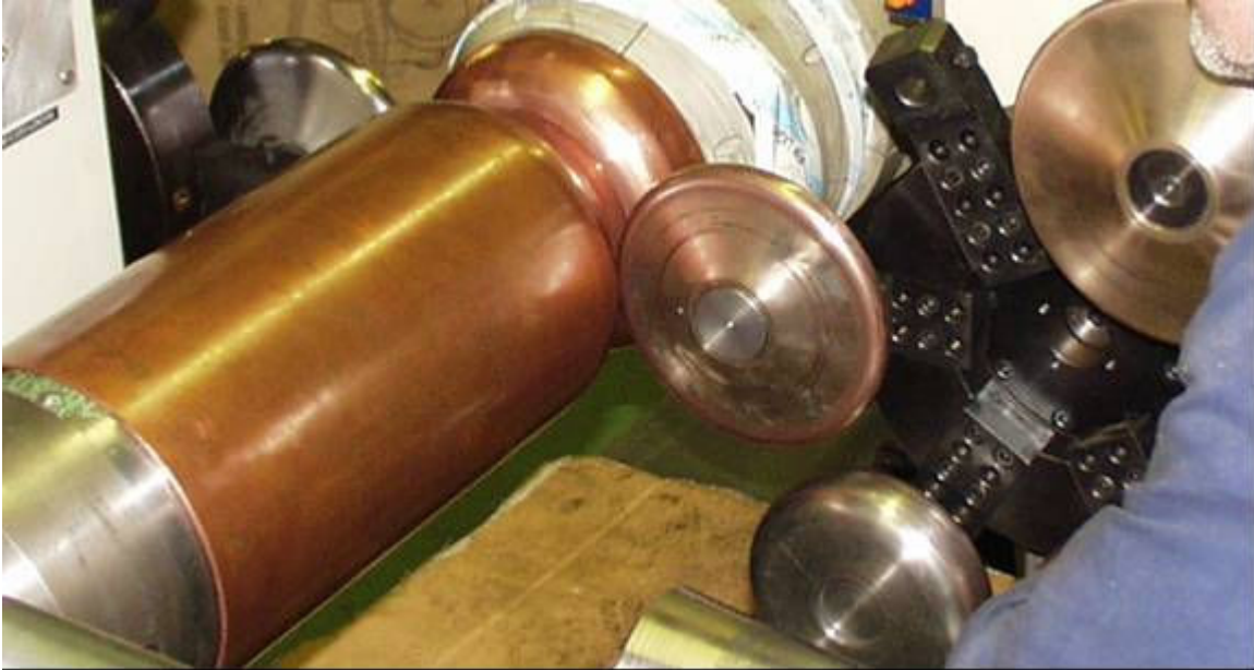
Fig. 3.1.3: Phase of the double turret necking process during the spinning parameter definition action.
