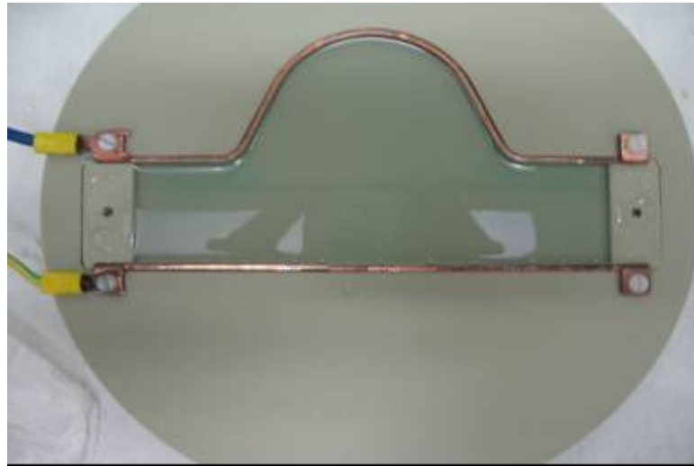
Fig. 6.2.1 Experimental Arrangement for magnetometric investigation of EP current distribution.
