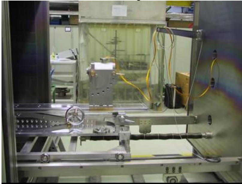
Figure 2.3.1: Motor box and current supply with Kapton© isolation
