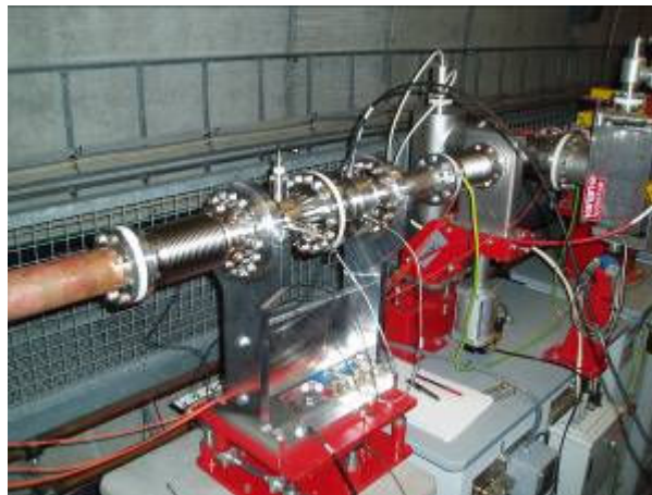
Figure 11.1.3b: Re-entrant cavity BPM and subsystem with hybrid couplers and phase shifters installed in the FLASH linac
