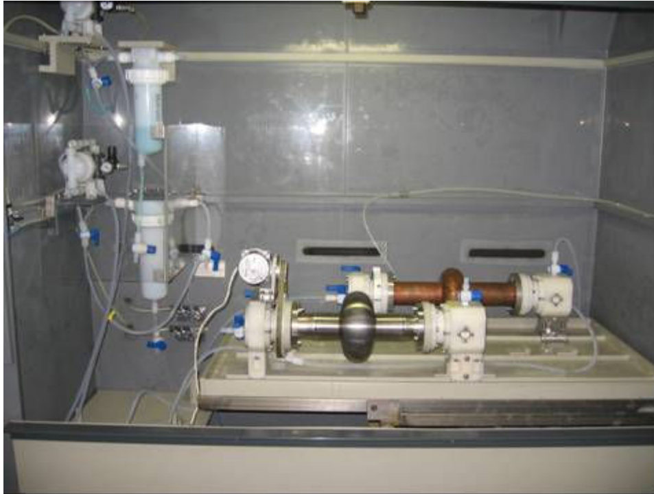
5.3.5 – The rotating cavity EP system built for the treatment of both Niobium and Copper.
