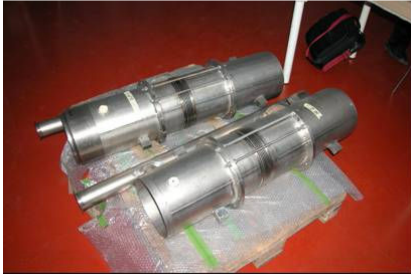
Figure 8.1.1: TTF cavities modified Helium tanks
