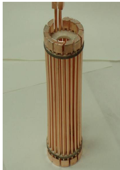
Fig.4.1.2. Distribution of magnetic field lines in the cross-section of the considered micro-droplet filter, and a general view of that filter prepared for the installation.
