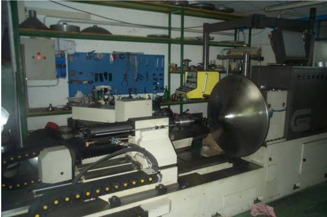
Fig. 3.1.1: The spinning lathe used for the fabrication of seamless cavity prototypes. The lathe had only one turret which held the rollers.
