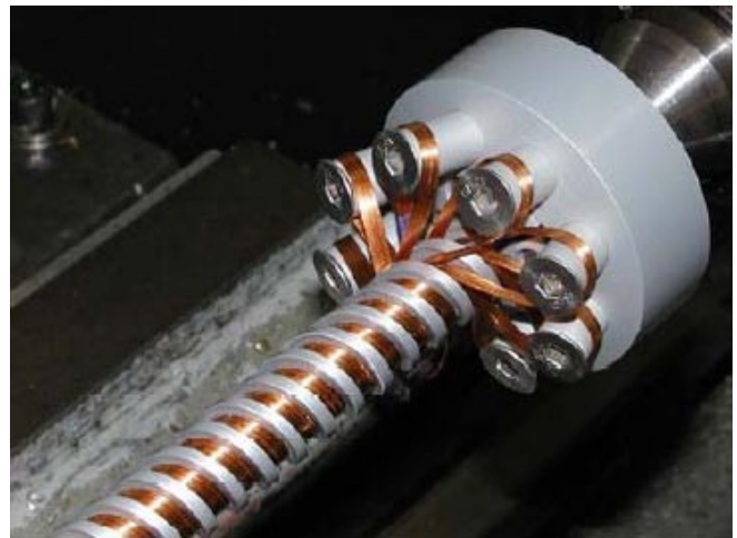
FIG. 9. (Color) Photograph of undulator winding showing the return pegs to allow for continuous winding.
