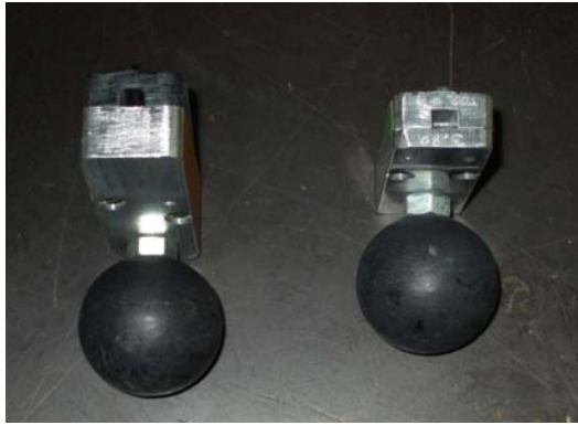
Fig. 20 Profile insertion tools were developed at ANL as well as at the other sites. This ANL tool compresses the fiber profile, and directs the compressed part into the slot between steel plates at the tile
