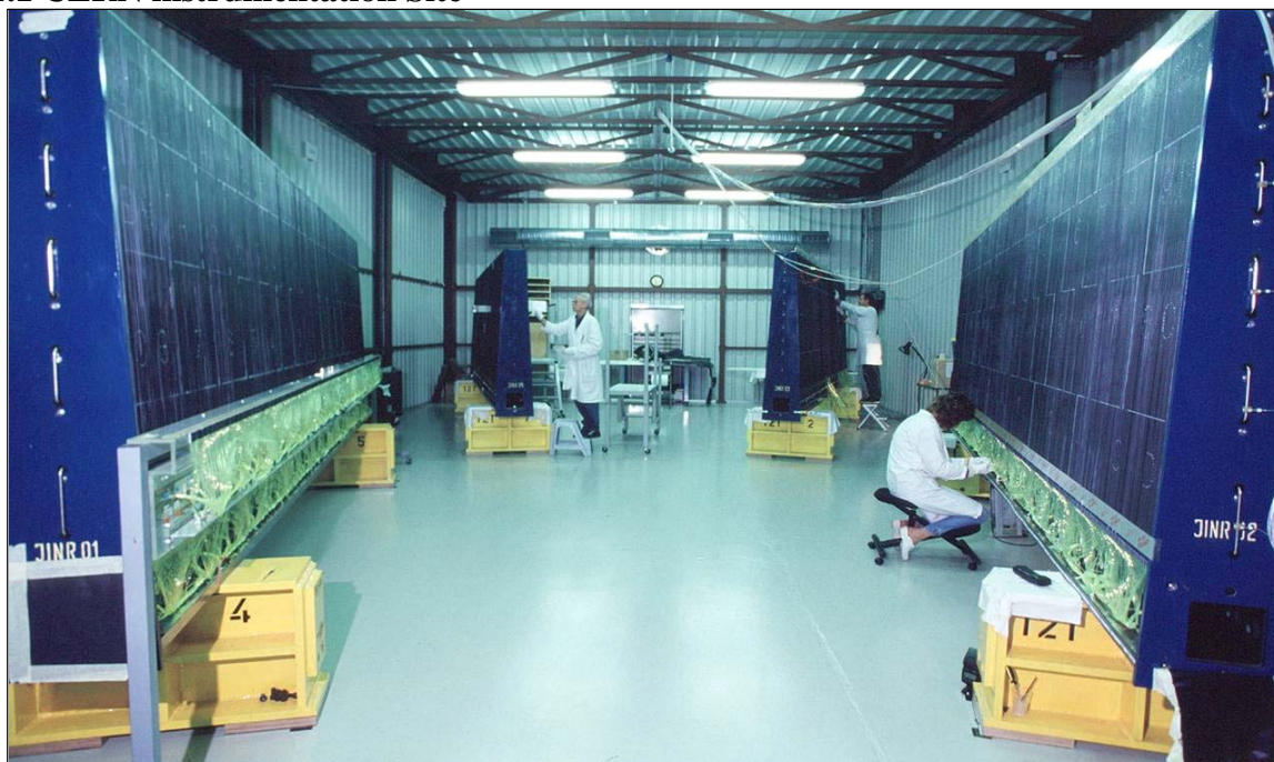
Fig. 7. The instrumentation room at the CERN Prevezin site. Four Barrel modules are at various stages of instrumentation, from tiles and fiber insertion to fiber routing and repairing. Calibration tubes to check the optical quality of with the ^{137}\text{Cs} source are seen on the front end-plates.
