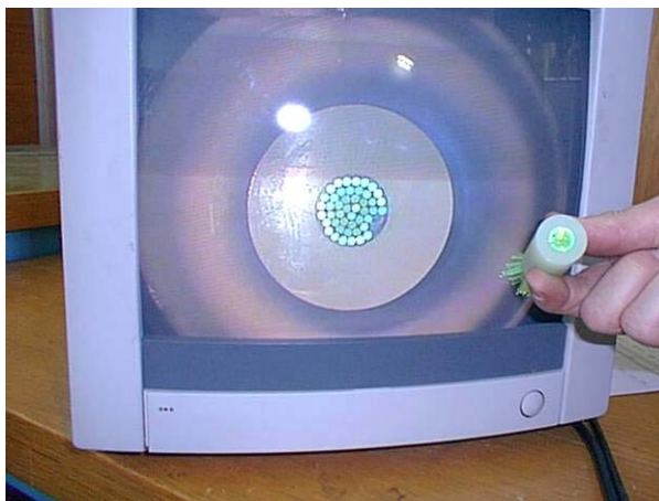
Fig. 15. Screen from a mini camera showing a polished Lucite tube with bundle of bright WLS fibers and dimmer points from two Teflon tubes, used to insert spare fibers if needed, at the edge of the bundle.
