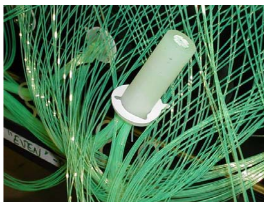
Fig. 10. A fiber bundle ready for being potted into a Lucite container.
