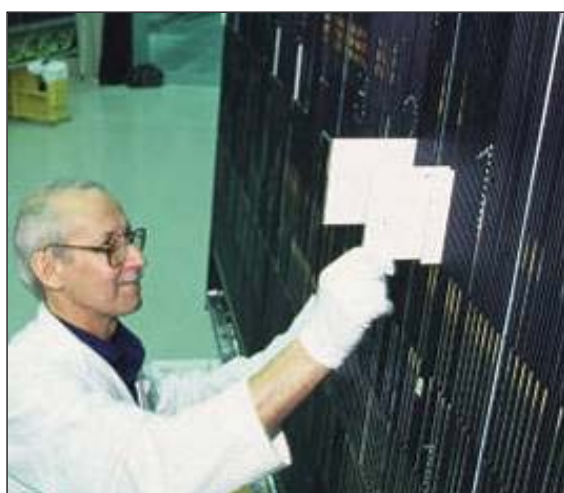
Fig. 8. Inserting tiles and profiles with fibers into a Barrel module
