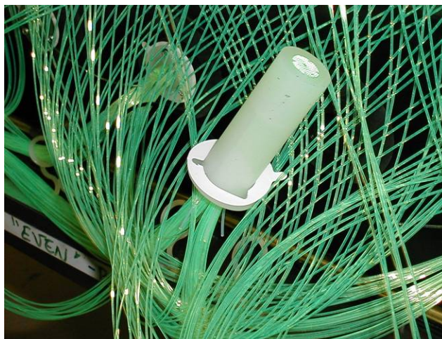
Figure 9. A fiber bundle ready for being potted into a Lucite container.
