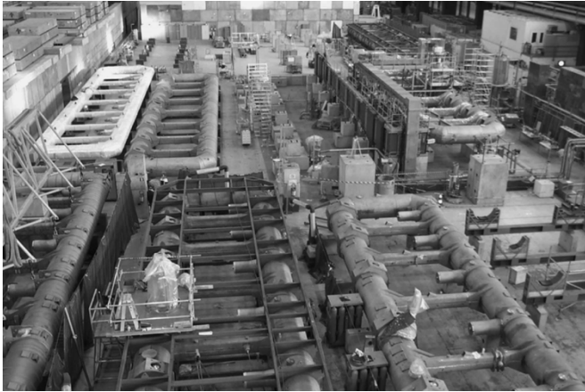
Fig. 2. View on the assembly and test area at a certain moment of assembly in February 2005. A few coils are already installed into the vacuum vessels. One cold mass is prepared for integration. One coil is in the X+ test bench. Being part of the production schedule a delay in the might affect the overall planning.
