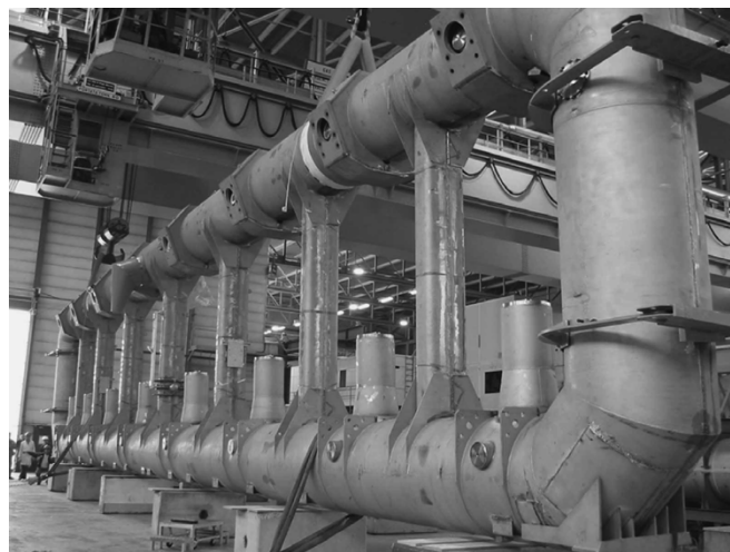
Fig. 1. The individual Barrel Toroid coil has passed the on-surface test in the ATLAS Magnet Test facility and is being prepared for the transport to the underground area of the ATLAS experiment.
