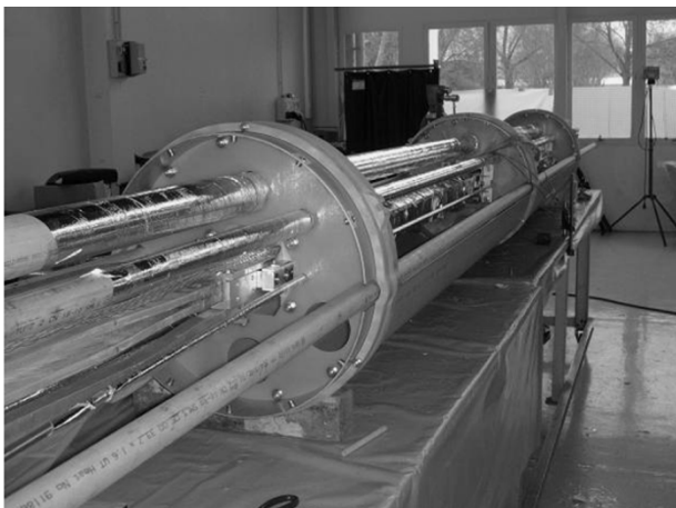
Fig. 4. Cold mass before the assembly of the thermal shields. He tubes are visible as well as the busbar on the center of the assembly.
