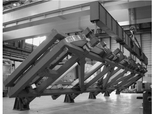
Fig. 2. A cold mass comprising one coil casing and two double pancake windings during a turn over operation.
