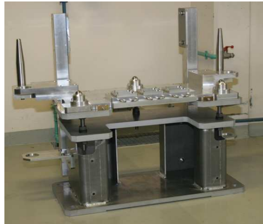
Figure 1: Photograph of an collimator base-support assembly, including lower plug-in and alignment plate.
