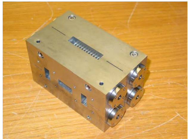
Figure 1: Photo of the assembled accelerating structure (HDX11mo) made out of 4 Molybdenum quadrants. Visible are the input and output coupler waveguides as well as the flanges to connect the water cooling pipes.
