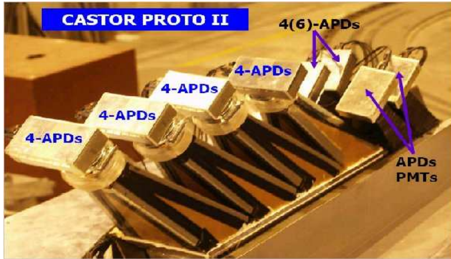
Fig. 4. Assembled prototype II on the moving table in the CERN/SPS H2 beam line. Only the APD readout units are shown.
