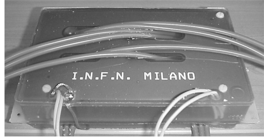
Fig. 6. View of an HV board when covered with STG with a shielding cover on the top (Cu shield is found just under the Solder Resist, where the Institution name is written).
