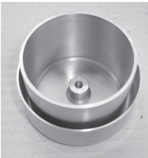
FIG. 3. Detail of the tuning cup before welding.
