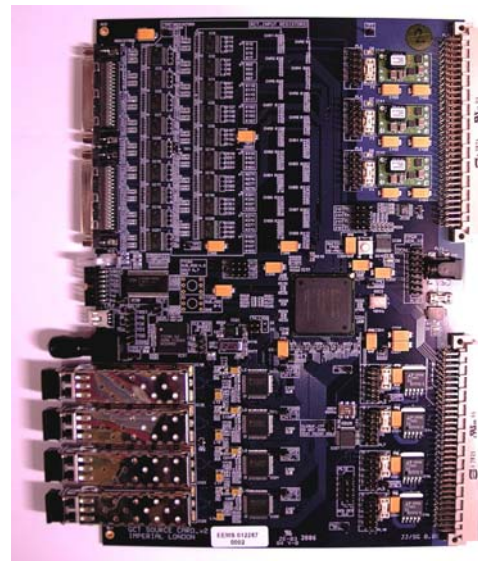
Figure 2: The Source card. The RCT inputs are visible in the top right of the picture. The 4 SFP cages are in the bottom right. All the signals are routed through a Xilinx Spartan 3 (XCS1000-5FG676C).
