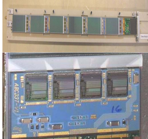
Figure 5: Stave with 6 sensors and the hybrid card.
