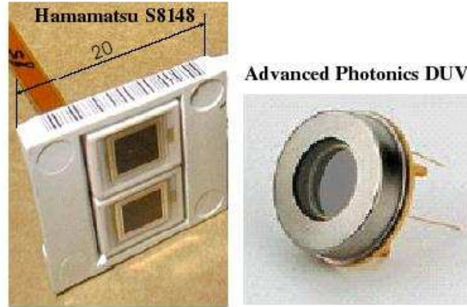
Fig. 8. The two types of APDs used in the beam test: Hamamatsu S8148 (left, 5 \times 5 \text{ mm}^2 , in a 2 \times 2 matrix with total 1 \text{ cm}^2 active area) and Advanced Photonix DUV (right, active area of 2 \text{ cm}^2 ).
