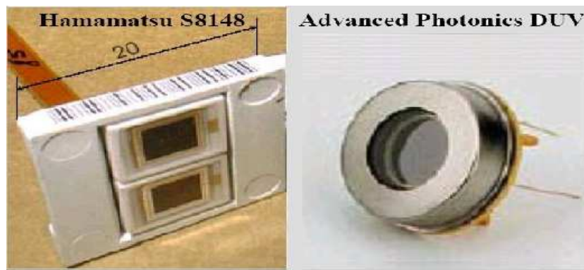
Figure 8: The two types of APDs used in the beam test: Hamamatsu S8148 (left, 5 \times 5 \text{ mm}^2 , in a 2 \times 2 matrix with total 1 \text{ cm}^2 active area) and Advanced Photonix DUV (right, active area of 2 \text{ cm}^2 ).
