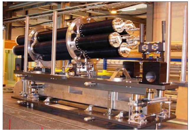
Fig. 5. CNGS target magazine consisting of five target units. Only the bottom unit is used, the other four are kept as spares.
