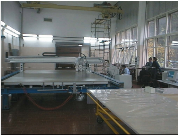
Figure 16: The Electrode Strip Production Line assembled in JINR-Dubna
