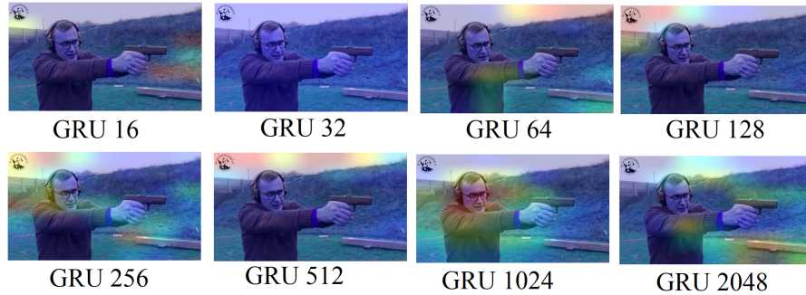
Figure 8: Activation map with variation of the number of neurons in the GRU Layer.
