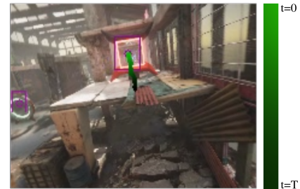
Fig. 1: MPC-predicted future pixel trajectory (Green) of a target pixel, the center of a gate. PixelMPC computes the optimal control which accomplishes a racing task and drives the target pixel to the center of the image.
